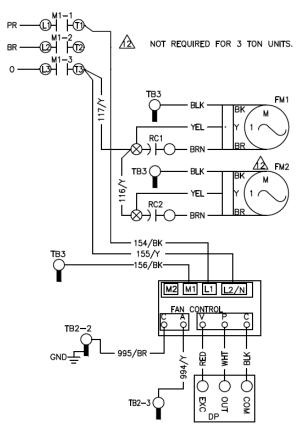
Note: Wiring numbers and colors may differ between nomenclature types, wiring should be as follows:
